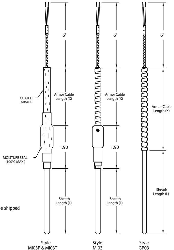
\*Note: GP thermocouples, manufactured using hollow tubing and wire, tend to be lower cost than MI, but cannot be bent in the field and are standardly designed for sensing temperatures below 500°F. MI thermocouples are more rugged than GP due to compacted magnesium-oxide powder insulation, can be bent in the field, and are appropriate for the temperature range of the sensor and sheath.
